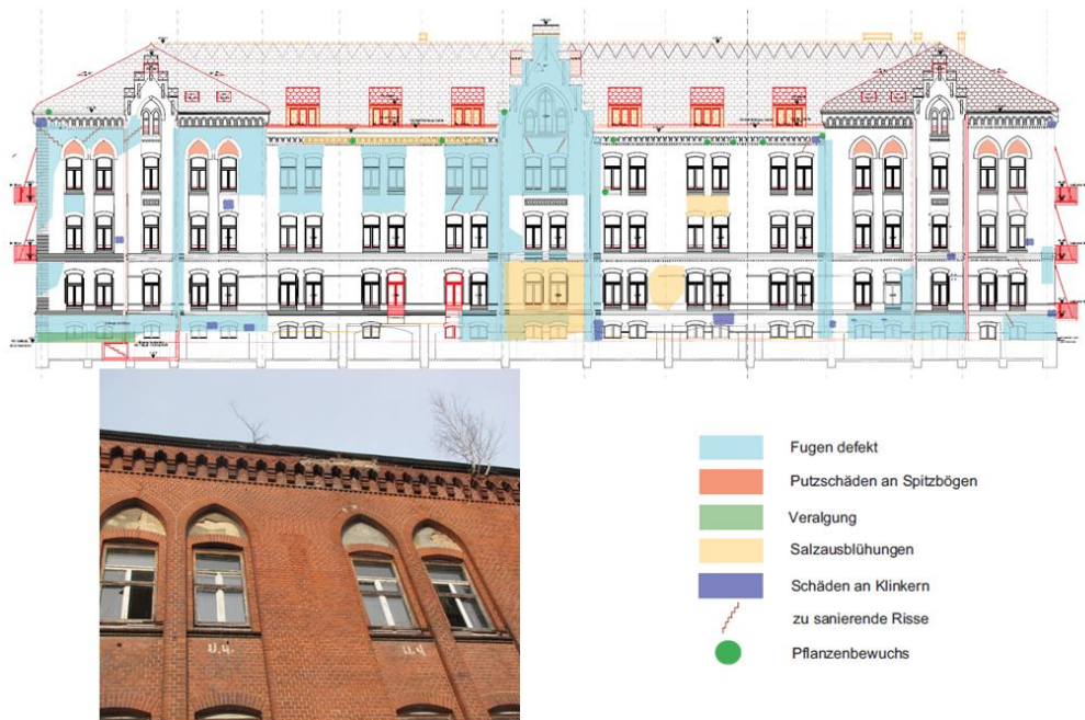
Fig. 2 Drawing with damage pattern found on a façade
