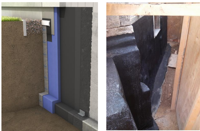
Fig. 25 Principle sketch for an external vertical seal (source: https://www.remmers.com/de/bauwerksabdichtung/neubauabdichtung ) and example of a design
