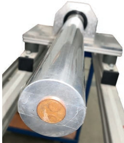
5ct coin as a pulse shaper at the input bar of the split-Hopkinson bar | Photo: Oliver Mosig
