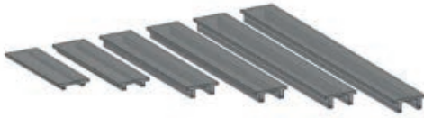
Comparative design of the double-T beams with span 6.0 m – 17.5 m | Graphic: Margarita Kondrakhina
