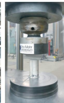
Kennwertermittlung an einer Betonprobe | Determination of characteristic properties on a concrete sample
