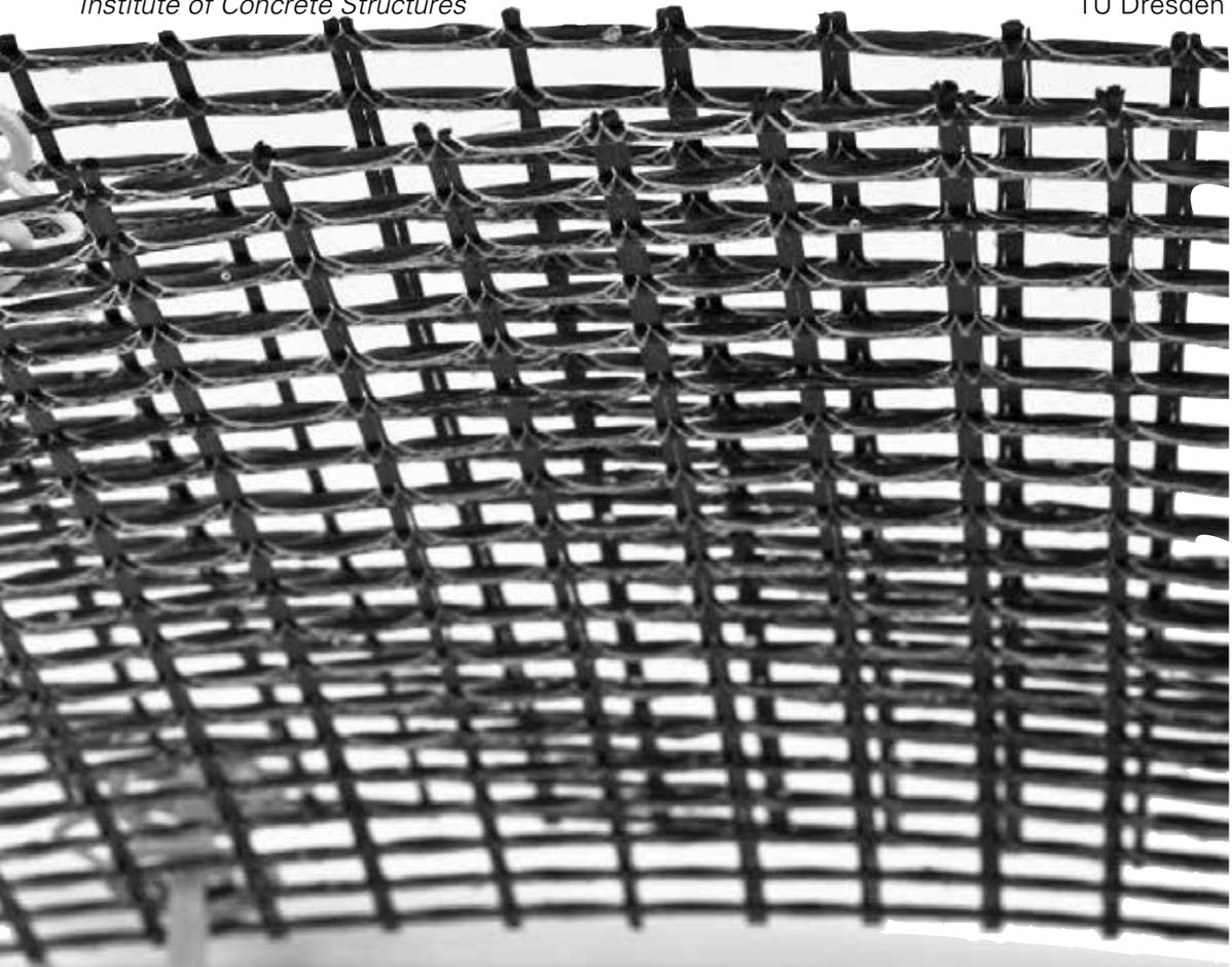
Textile reinforcement made of carbon yarn with spacers Photo: filmaton
