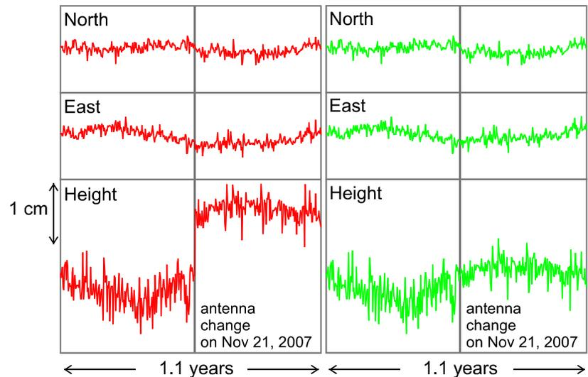
Fig. 5: Coordinate solution (L0+T) for Daun in the network of surrounding stations (Prüm, Mayen, Bernkastel-Kues) without (left) and with (right) application of phase maps (A) as shown in Fig. 4.
