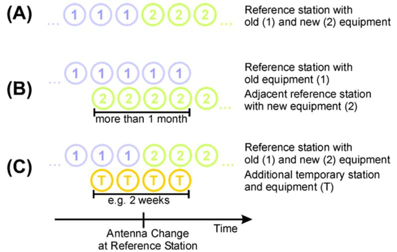
**Fig. 1:** Antenna change methods: (A) without any additional observations, most commonly used at CORS, (B) procedure recommended by the International GNSS Service (IGS) for its stations, (C) method proposed in this paper.
