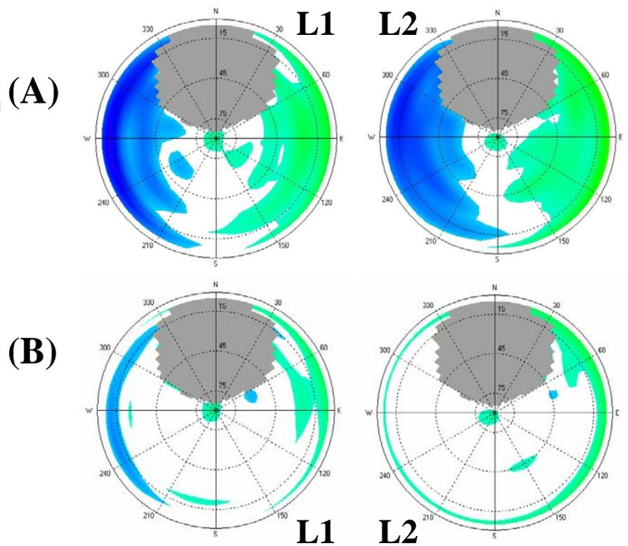
Fig. 4: Azimuth-elevation dependent observation corrections for reference stations Daun and Koblenz. (A) L1 and L2 phase maps to be used without any coordinate corrections, (B) phase maps reduced by the effects of the coordinate corrections (cp. Tab. 2)
