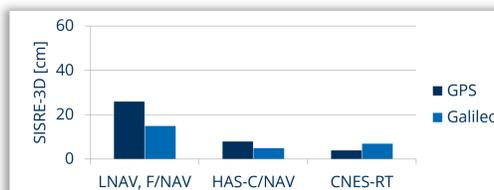
Fig. 4: Accuracy of real-time orbit corrections as signal in space range errors 3D (SISRE-3D)
