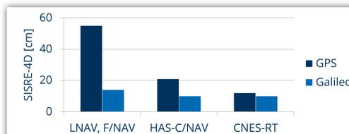
Fig. 5: Accuracy of real-time orbit and clock corrections as signal in space range errors 4D (SISRE-4D)
