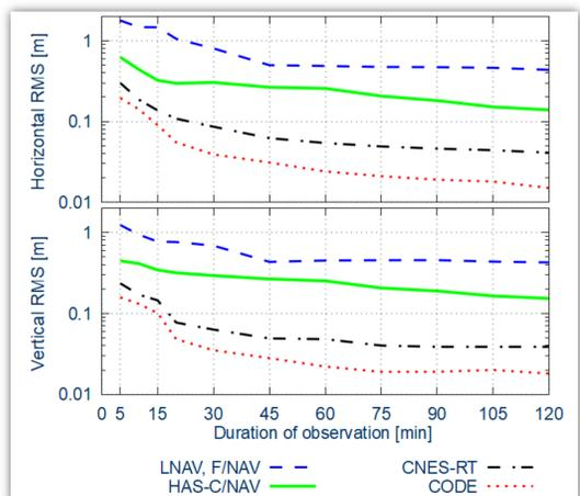
Fig. 6: Accuracies as root mean square values (RMS) of kinematic float-PPP solutions depending on the duration of observation
