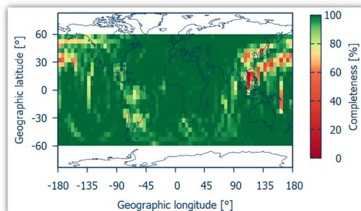
Fig. 2: Spatial availability of Galileo HAS corrections mapped to the satellites' ground tracks
