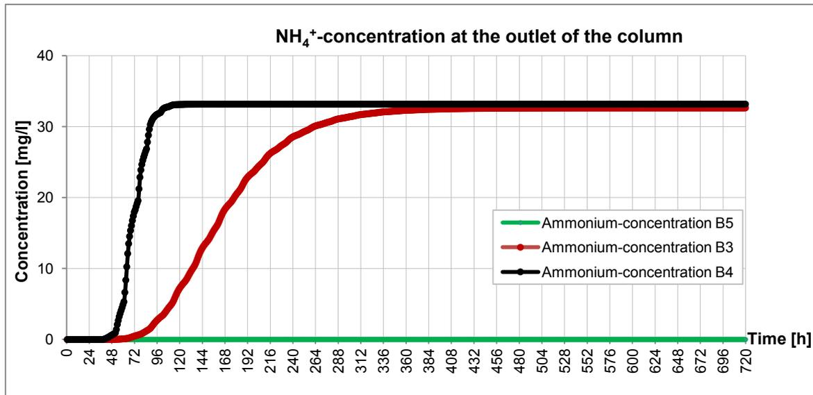
Figure 8. Computed Ammonium- concentration using PCSiWaPro<sup>®</sup> for the three studied soils B3, B4 and B5 during 30 days of simulation
