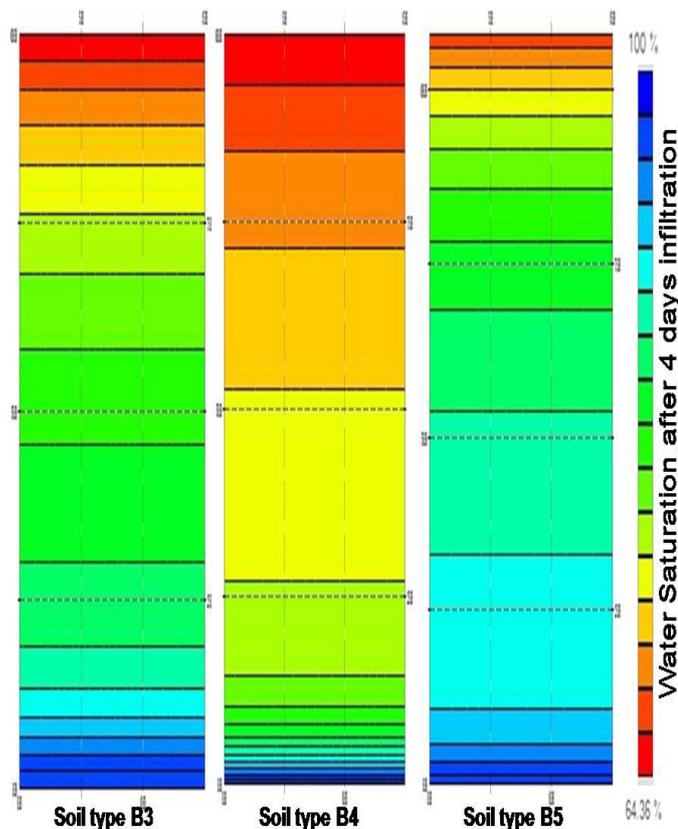
Figure 5. Distribution of water saturation after 4 days of infiltration for the investigated soils
