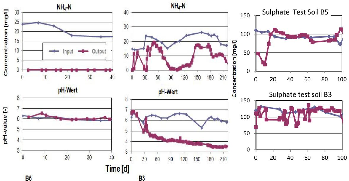
Figure 7. Measured results pH-value and  $\text{NH}_4\text{-N}$ -concentration for the soils B3 and B5 (left) and sulphate analysis for B5 and B3 (right)
