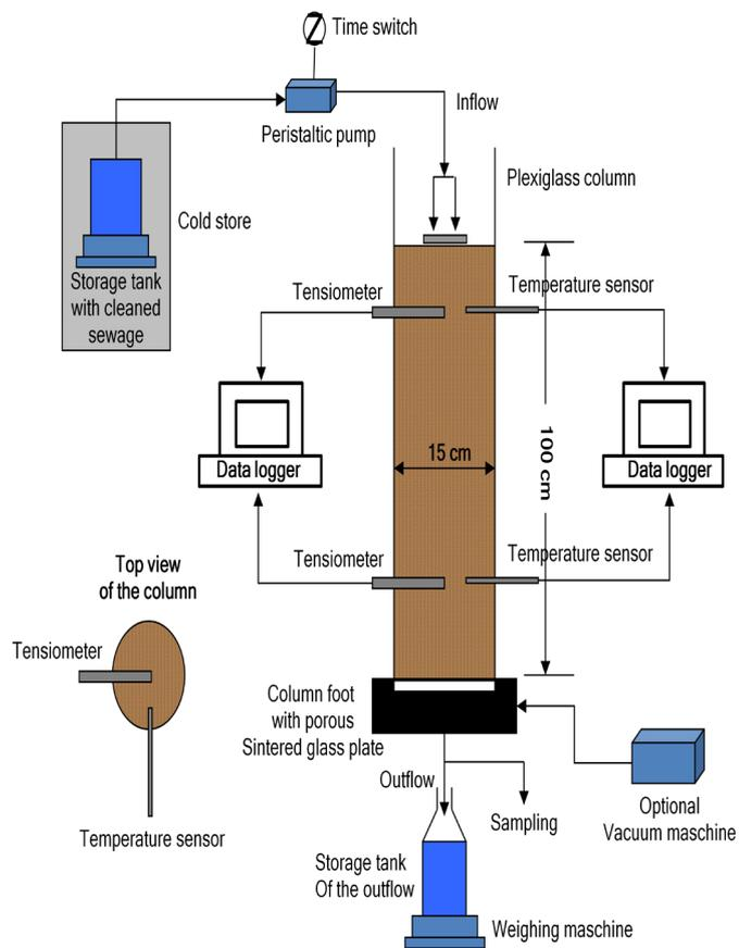
Figure 2. Setup of the soil-column experiment (ESEK, 2011)
