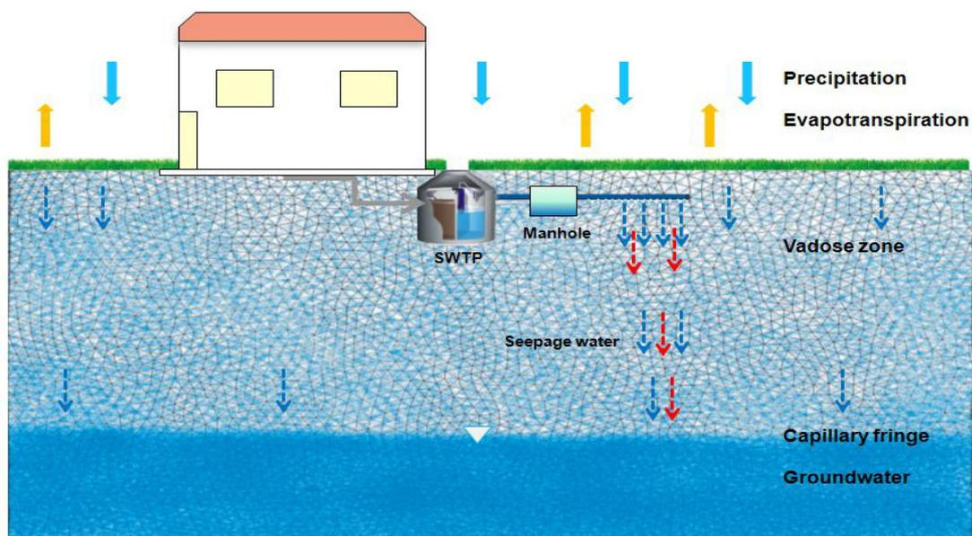
Figure 1. schematical representation of the investigated model and the parameters of soil water balance
