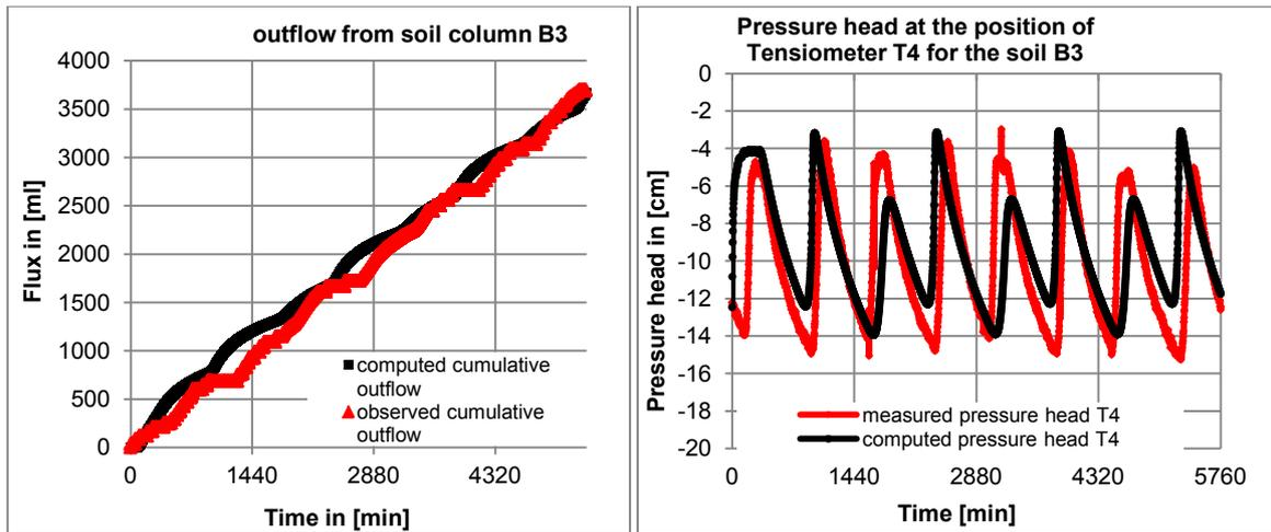
Figure 6. Comparison between measured and computed values (drain water (outflow), pressure head) for B3
