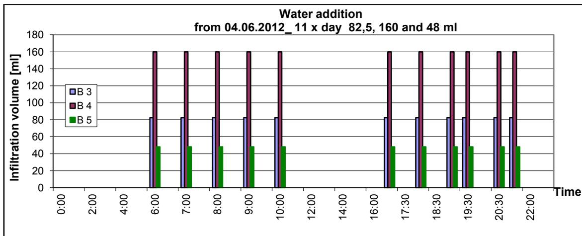
Figure 3. Infiltration rates of sewage for the three investigated soils B3, B4 and B5
