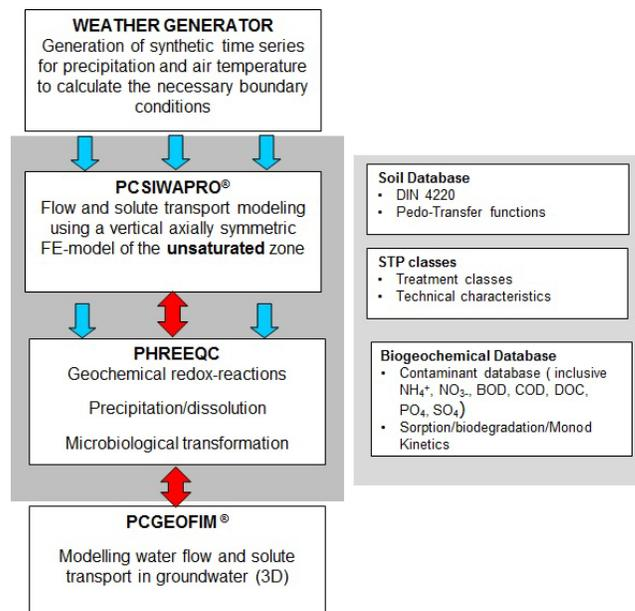
Figure 2. Coupling of numerical simulation codes and databases.
