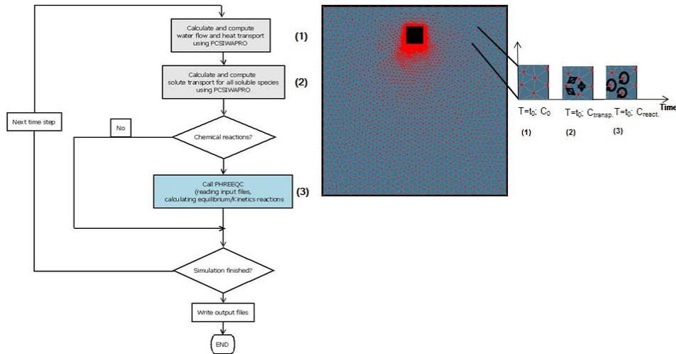
Figure 3. Coupling between the PCSiWaPro<sup>®</sup> and PHREEQC in a 2D cross-section.
