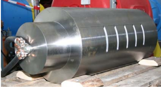
Figure 3: 2-pole turbine generator rotor mock-up with 5 cross slits machined into the pole
