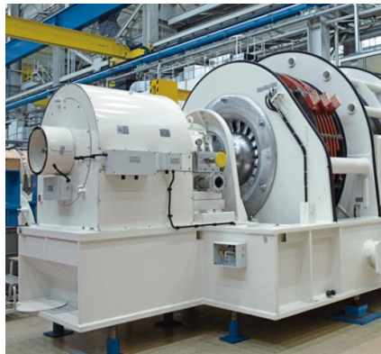
Fig. 1: Final assembly of a turbo generator [Siemens Generator Plant Erfurt]
