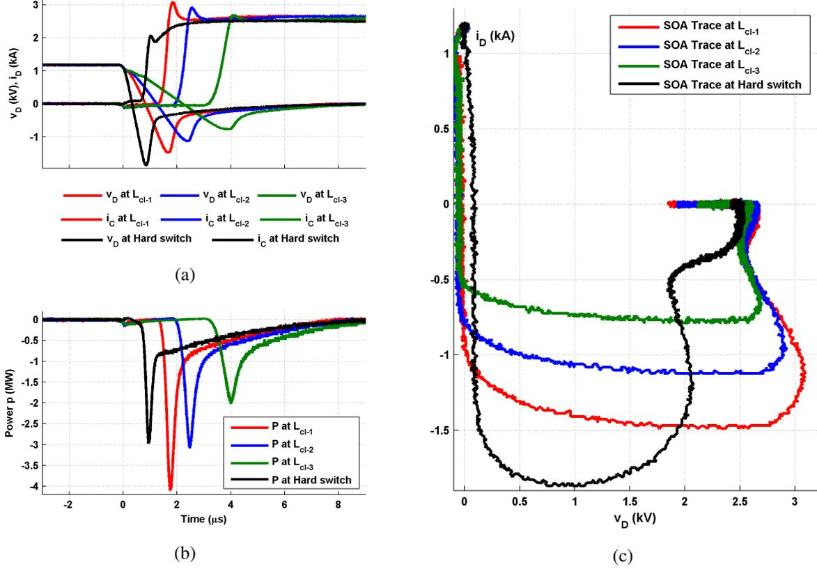
Figure 5: Diode turn-off behavior (a) waveforms, (b) peak power, (c) Safe Operating Area trajectories ( $T_j = 125^\circ\text{C}$ ,  $V_{DC} = 2.5\text{ kV}$  and  $i_C = 1.2\text{ kA}$ )
