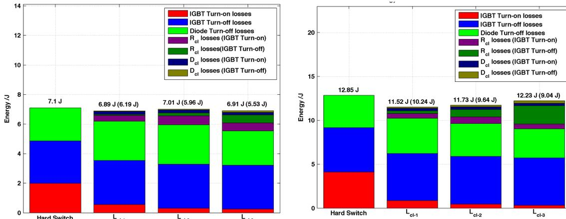
Figure 6: Semiconductor and clamp switching losses ( $V_{dc} = 2.5$  kV,  $T_j = 125$  °C,  $i_C = 600$  A)
