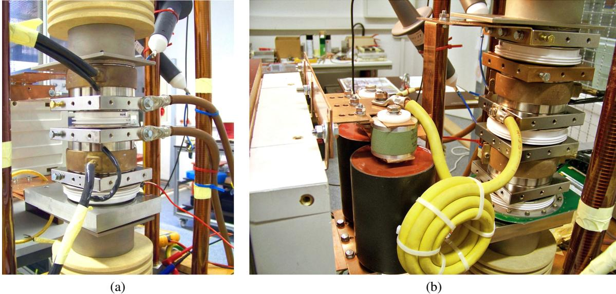
Figure 2: Experimental setup (a) IGBT stack for hard switching, (b) stack with clamp circuit
