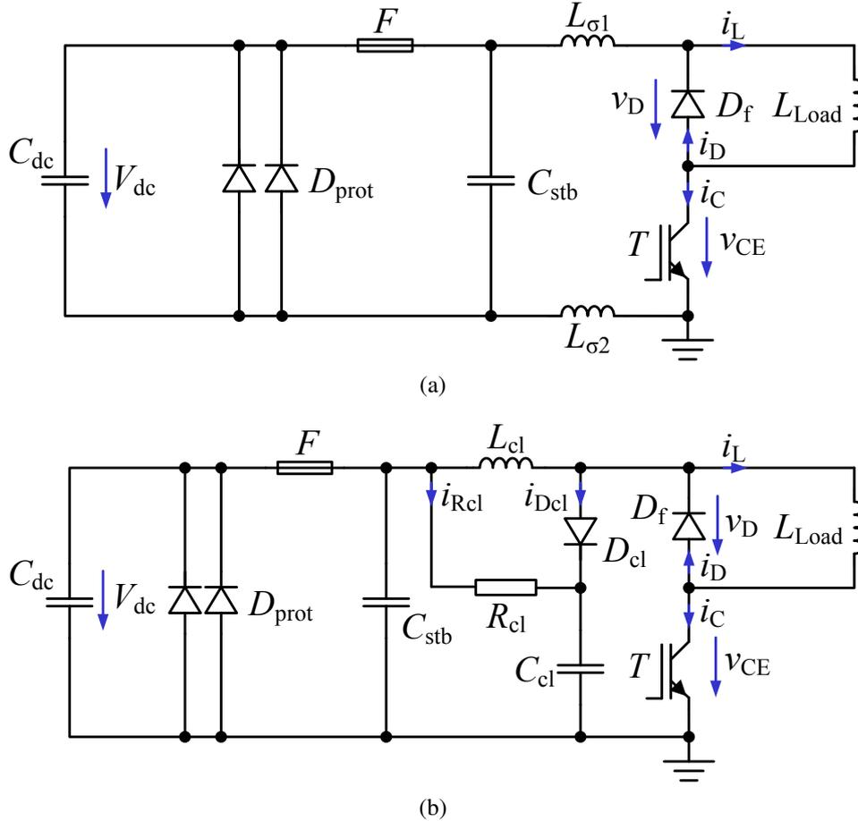
Figure 1: Test bench schematic diagram for (a) hard switching and for (b) soft switching with clamp circuit
