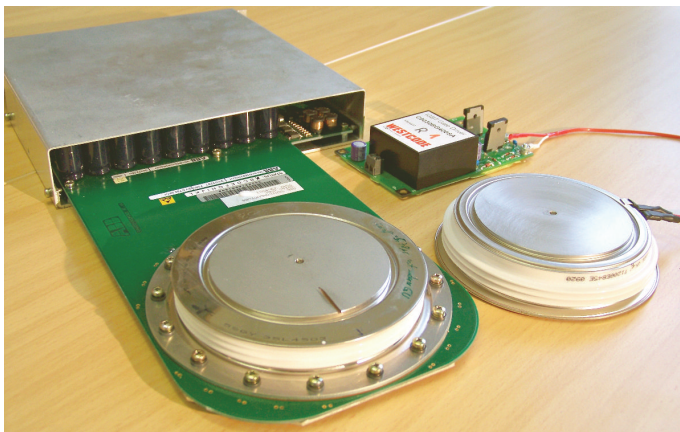
Fig. 3. IGCT 5SHY 35L4503 (left) and IGBT T1200EB45E with gate unit (right)
