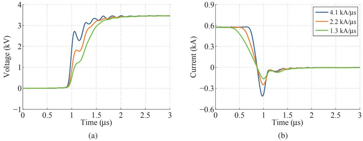
Figure 12: Measured voltage and current waveforms for diode turn-off at different  $di/dt$  with an RC snubber:  $C = 9.4 \text{ nF}$ ,  $R = 4.7 \Omega$  for  $di/dt = 1.3, 2.2 \text{ kA}/\mu\text{s}$ ;  $C = 14.1 \text{ nF}$ ,  $R = 4.7 \Omega$  for  $di/dt = 4.1 \text{ kA}/\mu\text{s}$  ( $V_{dc} = 3.5 \text{ kV}$ ,  $I_D = 600 \text{ A}$ ,  $\vartheta_j = 25^\circ\text{C}$ )
