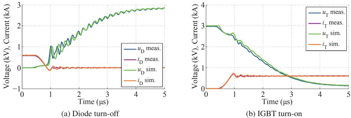
Figure 5: Comparison measurement/simulation at calibration point ( $V_{dc} = 3 \text{ kV}$ ,  $I_L = 600 \text{ A}$ ,  $\vartheta_j = 25^\circ\text{C}$ ,  $R_{g,on} = 4.1 \Omega$ )
