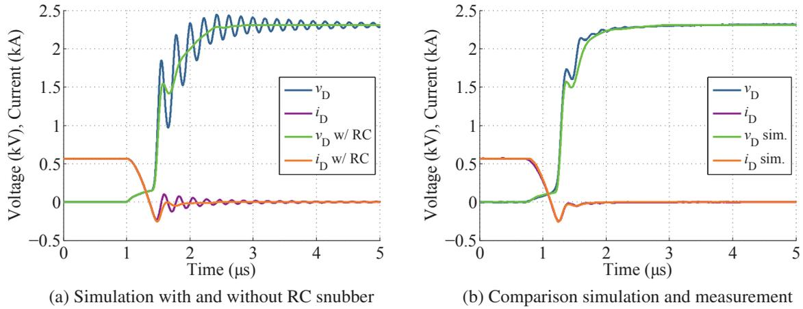
Figure 11: Effect of an RC snubber circuit connected to the diode ( $C = 9.4 \text{ nF}$ ,  $R = 4.7 \Omega$ ,  $V_{dc} = 2.3 \text{ kV}$ ,  $I_D = 600 \text{ A}$ ,  $di/dt = 2.2 \text{ kA}/\mu\text{s}$ )
