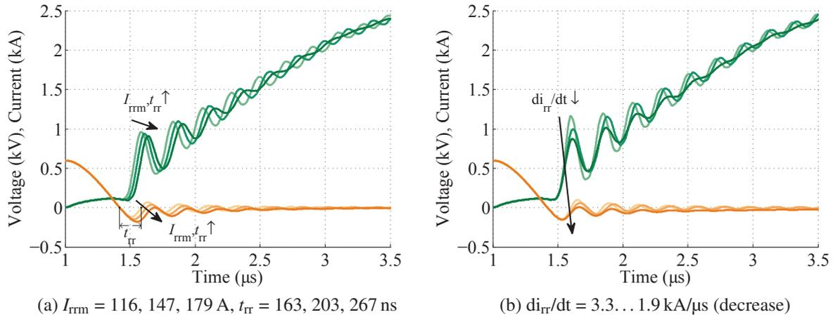
Figure 9: Influence of the simultaneous variation of reverse recovery current peak  $I_{rrm}$  and duration  $t_{rr}$  (a) and variation of the current change rate after the reverse recovery peak  $di_{rr}/dt$  (b) in the oscillations, green: voltage, orange: current ( $V_{dc} = 3 \text{ kV}$ ,  $I_L = 600 \text{ A}$ ,  $R_{g,on} = 4.1 \Omega$ ,  $\vartheta_j = 25^\circ\text{C}$ )
