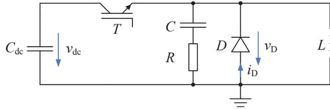
Figure 10: Test bench with an RC snubber added to the diode
