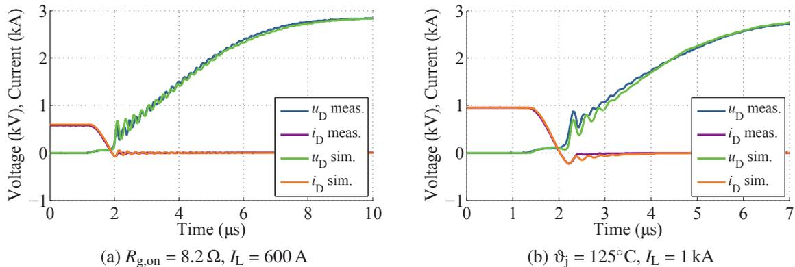
Figure 7: Comparison measurement/simulation of the diode turn-off transient at a different  $R_{g,on}$  and junction temperature  $\vartheta_j$  ( $V_{dc} = 3$  kV)
