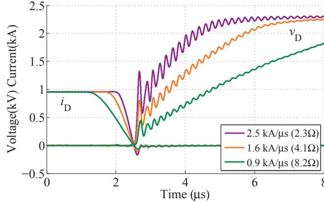
Figure 1: Oscillations during the diode turn-off transient for different  $di/dt$  (IGBT gate turn-on resistance) values (2.4 kV, 1 kA, 25°C,  $di/dt = 0.9 \dots 2.5$  kA/ $\mu$ s)
