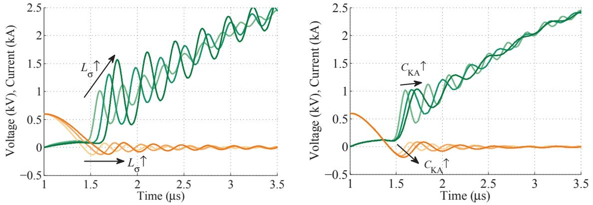
(a) Stray inductance  $L_\sigma = 106, 212, 318$  nH (increase) (b) Diode's junction capacitance  $C_{KA} = 1 \dots 3C_{KA,ref}$
