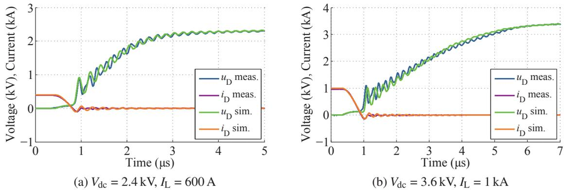
Figure 6: Comparison measurement/simulation of the diode turn-off transient at different  $V_{dc}$  values ( $\vartheta_j = 25^\circ\text{C}$ ,  $R_{g,on} = 4.1 \Omega$ )
