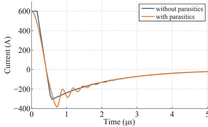
Figure 4: Comparison of the simulated reverse recovery current waveform with and without the effect of circuit parasitics
