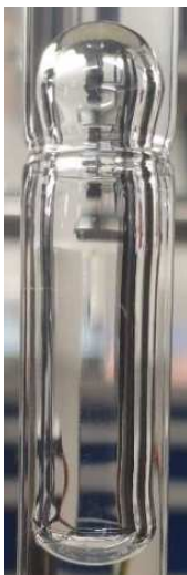
Fig 1: Taylor bubble in glas tube with constriction
