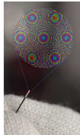
Lensless holographic endoscope: Magnification shows the light phase on the fiber for far field focusing
