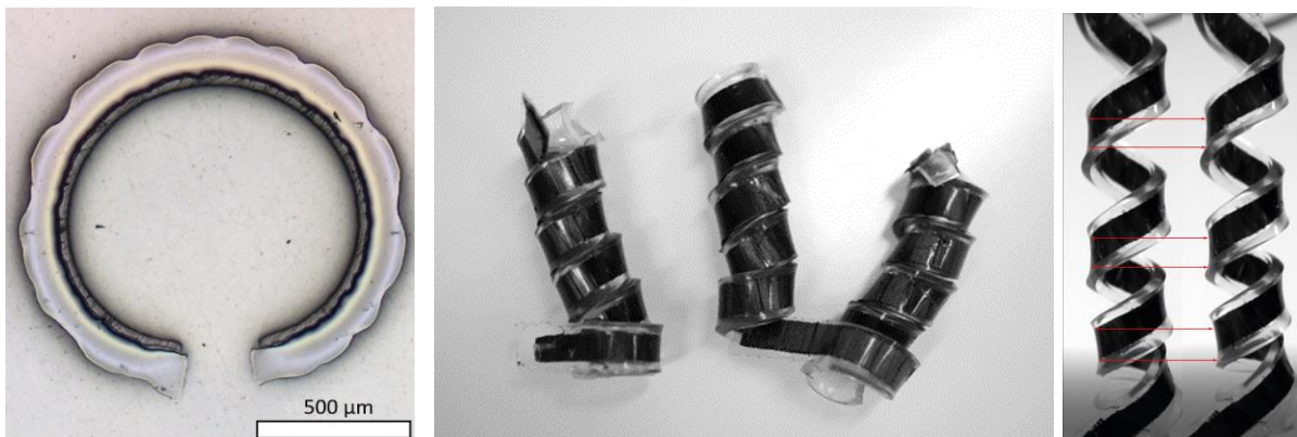
Helix-shaped dielectric actuator [1-3]
