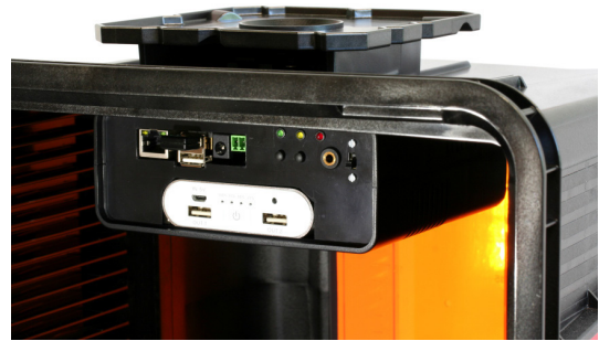
Fig. 3: Measurement device built into a FOUP
