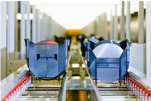
Fig. 2: Conveyor based transport system of a 200mm production line
