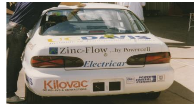
35 kWh Zn/Br race car ~1994 © Gerd Tomazic Roth, Noack, Skyllas-Kazacos, Flow Batteries, Wiley-VCH 2022
