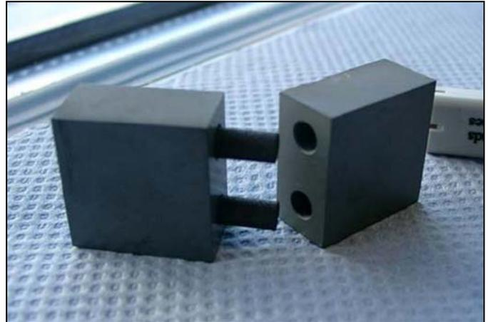
**Figure 5** Graphite bridges in SiC-body
