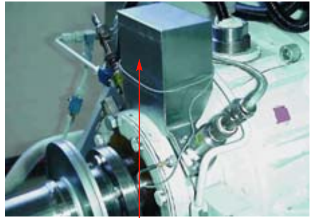
3 Example of a successful passive detuning: gearbox test bench with additional mass applied (RUAG).
