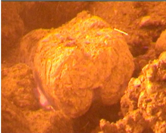
Fig. 5. Biomass briquette, burnout zone of the grate.
