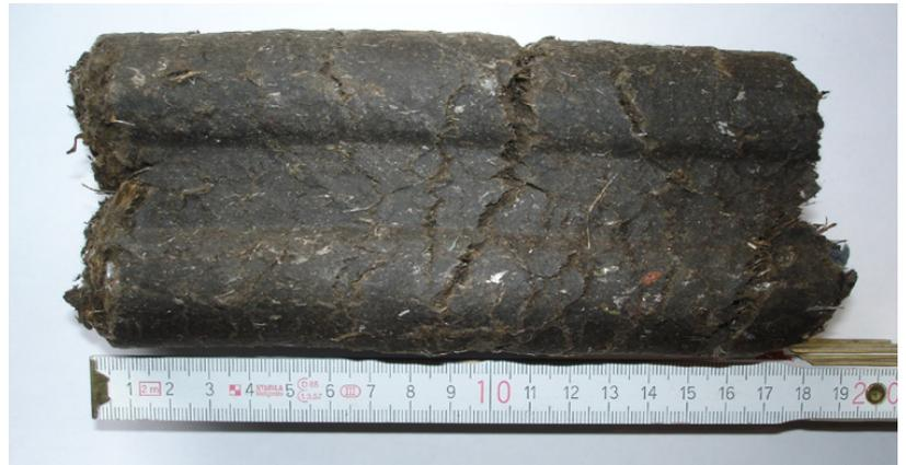
Fig. 4. *Biomass briquette, longitudinal view.*
