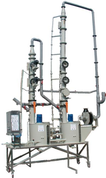
Figure 11: Wet Flue Gas Desulphurisation Scrubber test facility
