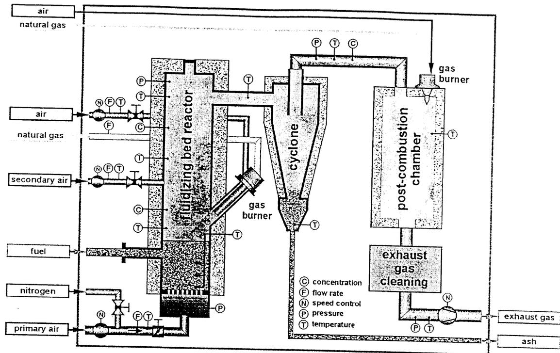
Figure 6: Flow chart of the fluidized bed reactor with post-combustion chamber.
