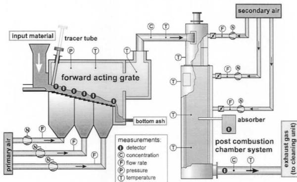
Fig. 1. Pilot plant and detector positions.
