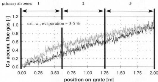
Fig. 3. Normalised Cu amount detected in flue gas scrubber after the pulsed addition of Cu tracer at position 0. Accumulation is monitored while tracer is transported along the grate (0.0 to 2.0 m). oxi.: oxidizing conditions; w: water content of waste.
