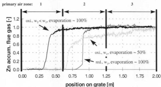
Fig. 4. Normalized Zn amount detected in flue gas scrubber after the pulsed addition of Zn tracer at position 0. Accumulation is monitored while tracer is transported along the grate (0.0 to 2.0 m). oxi.: oxidizing conditions; red.: reducing conditions (gasification); w: water content of waste.
