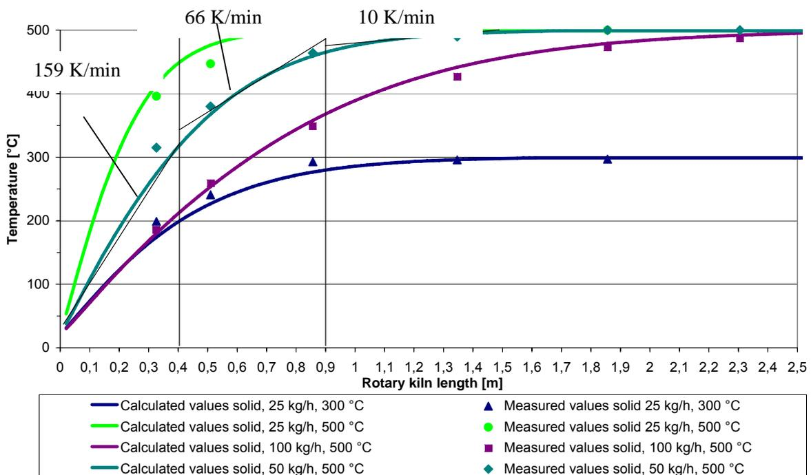
**Fig. 4:** Solid temperature profile ( $\Delta m/\Delta t = 0$ )
