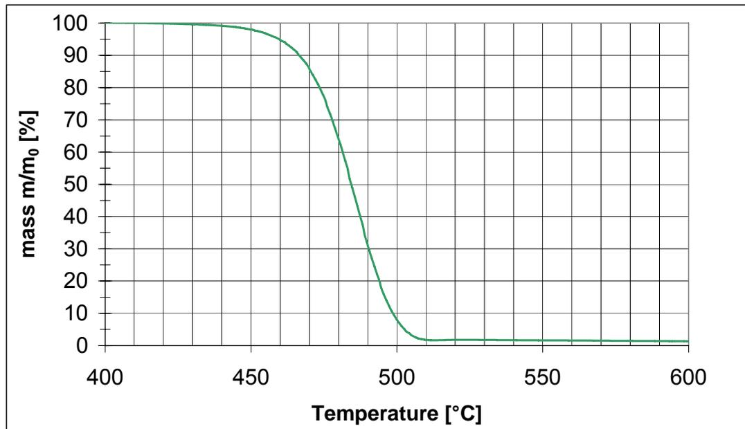
**Fig. 5:** Result from an investigation with the thermobalance with PE at a heating rate of 10 K/min
