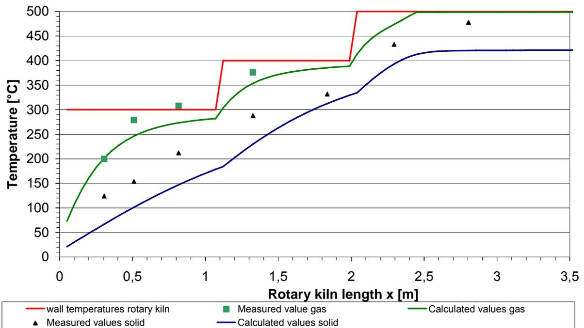
**Fig. 6:** Calculated and measured temperature profiles of solid and gas phase with a staging of the wall temperatures of 300/ 400/ 500/ 500 °C with 90 kg/h sand and 10 kg/h PE
