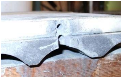
Fig. 8. JuSyS ® SL-plate with holes to measure the temperature gradient.
