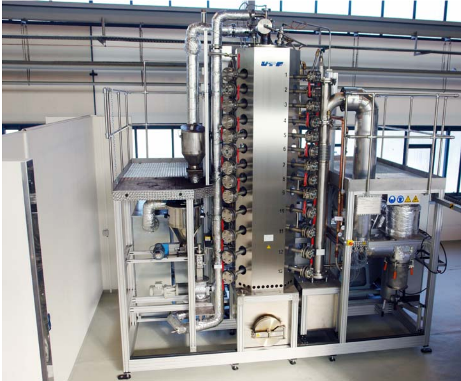
Figure 4: 50 kW th pulverised coal oxyfuel combustion test facility at the TU Dresden
