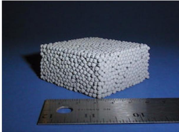
Figure 5. Sintered titanium aluminide hollow sphere structure, fabricated from 3 mm diameter spheres.
