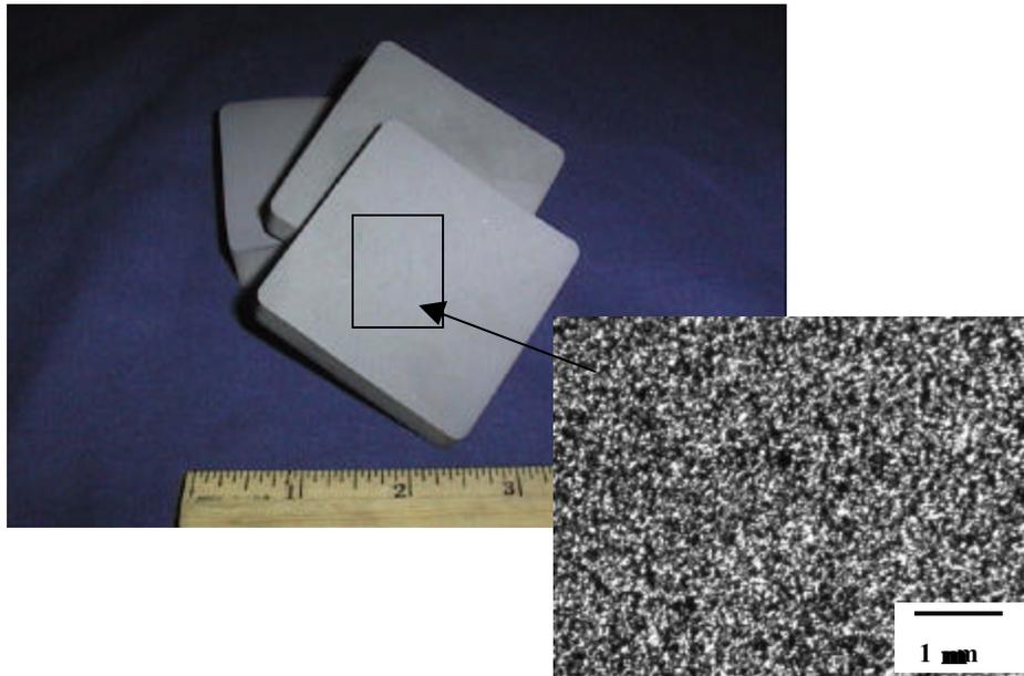
Figure 9. Reaction sintered Ti-Al plates with a close-up of the as-sintered surface (inset).
