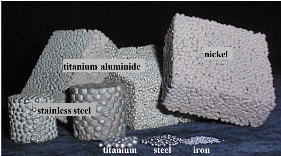
Figure 2. Examples of hollow sphere structures in various compositions.
