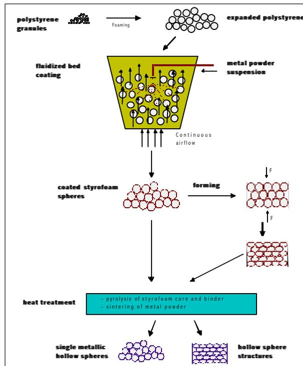
Figure 1. Schematic view of the process to produce hollow metal spheres.
