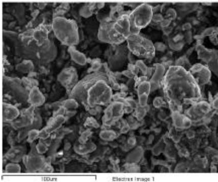
Figure 7. Al powder ( $\sim 75\mu m$ ) from Eckart America, L.P. used in the production of reactively sintered Ti-Al components.
