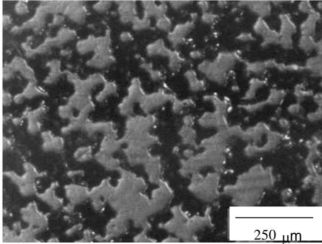
Figure 10. Polished cross-section of reactively sintered Ti-Al specimen (porosity ~ 54 volume %).
