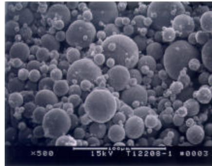
Figure 8. Ti powder ( $\sim 45\mu m$ ) from Pyrogenesis Inc. used in the production of reactively sintered Ti-Al components.
