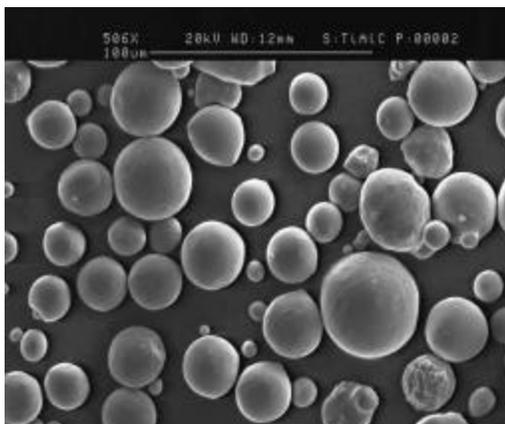
Figure 3. Pre-alloyed titanium aluminide powder from Crucible Research (506X)
