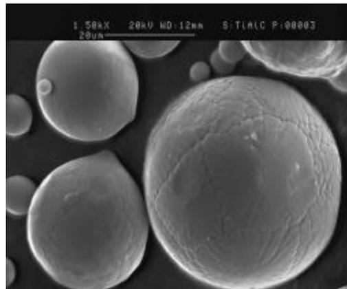
Figure 4. Pre-alloyed titanium aluminide powder from Crucible Research (1500X).
