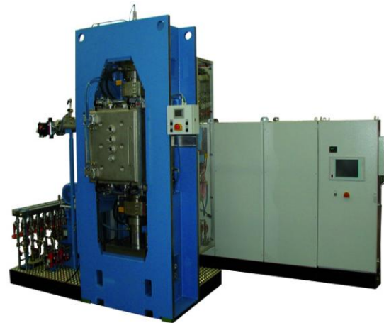
Figure 1. Aluminium pre-compacts ( \varnothing 75mm, h 85mm, 99,3% theoretical density) consolidated by SPS using the FCT-HP D 250 of FCT Systeme GmbH, Germany.
