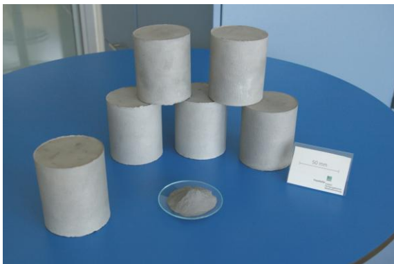
Figure 1. Aluminium pre-compacts ( \varnothing 75mm, h 85mm, 99,3% theoretical density) consolidated by SPS using the FCT-HP D 250 of FCT Systeme GmbH, Germany.
