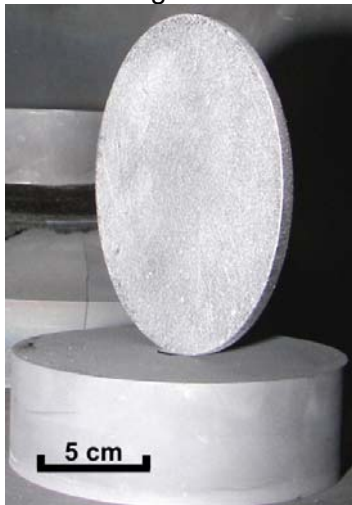
Figure 1: Sintered Body with a diameter of 150 mm and a height of 5 mm of a tungsten-graphite composite with 70 vol. % graphite.
