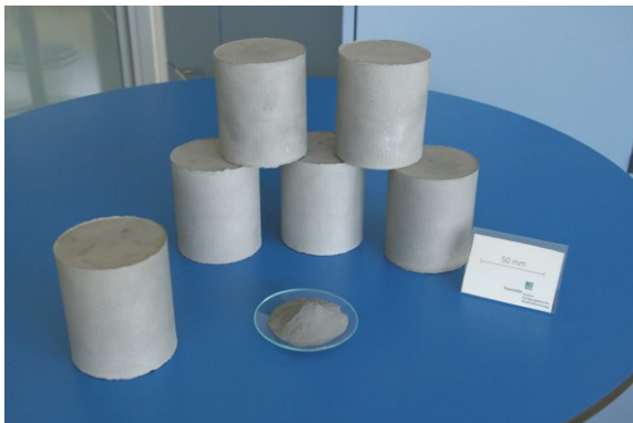
Figure 1. Aluminium billets ( \varnothing 75mm, h 85mm, 99,3% theoretical density) consolidated by SPS using the FCT-HP D 250 of FCT Systeme GmbH, Germany.
