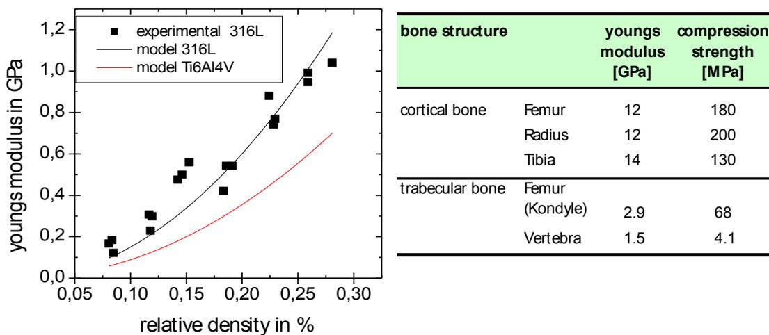
**Figure 5.** Mechanical properties of open cell metal foam (316L) in comparison to different types of bone
