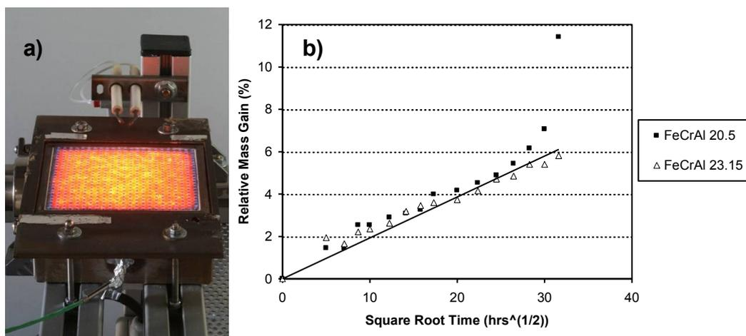
**Figure 3.** Burner test rig with IFAM fiber burner plate (Fig. a) and relative mass gain over time due to oxidation in air at 1000 °C for sintered fiber structures with a mean porosity of 75 % and different aluminum contents (Fig. b)
