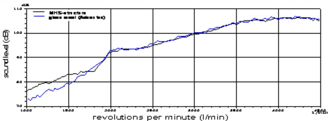
**Figure 8.** Sound level of Stainless Steel (316L) metal hollow sphere structures as a function of the revolution of a hot engine (BMW 2.4 TDI).
