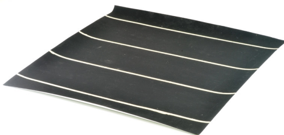
CNT-modified heating element with adapted electrical and thermal properties.
