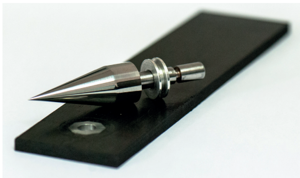
Fig. 01: FRP specimen with embedded insert and pin tool.
