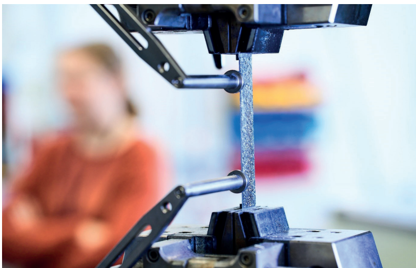
Tension test with fiber-reinforced plastics.
