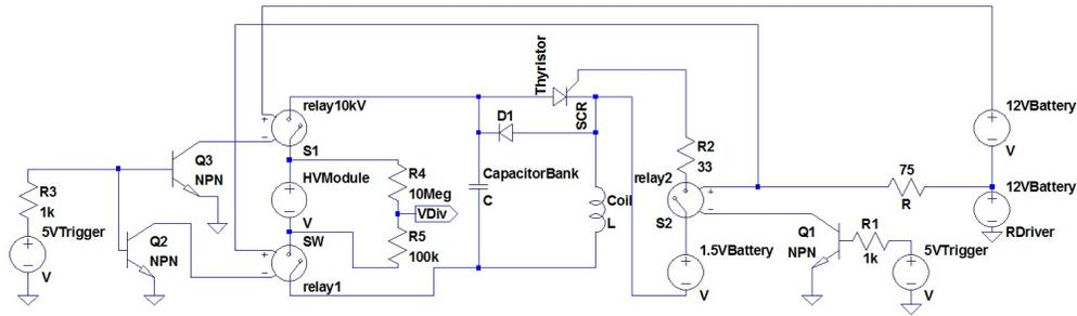
Figure 4. Schematic of the small-scale impulse generator's circuit
