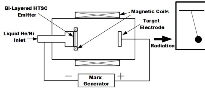
Figure 1. Schematic of Podkletnov's experimental setup<sup>1</sup>
