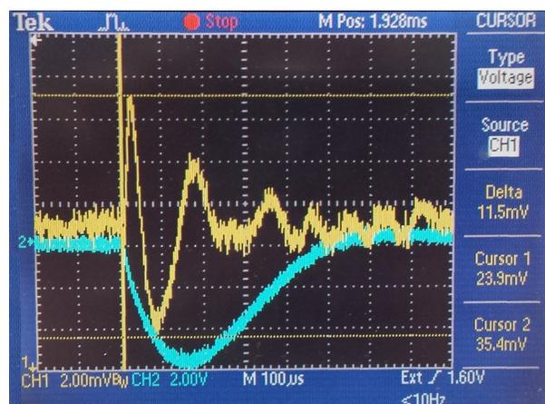
Figure 10. Anomalous accelerometer readout during a 500 V DC discharge through an YBCO disc below its critical temperature. CH1 is the accelerometer output (1.2 V/g) and CH2 is the current output (1 V/1 kA)
