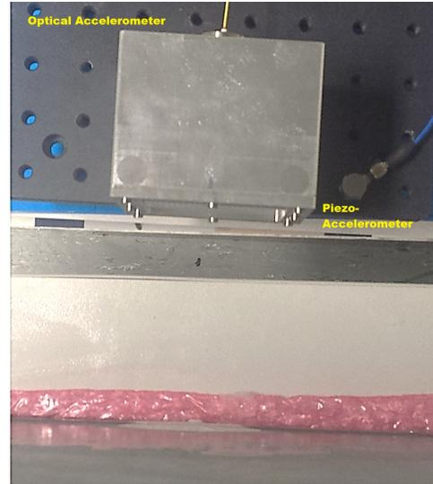
**Figure 14.** The optical accelerometer (top-center) facing the cryostat and the piezo-accelerometer (top-right) placed vertically for the reference measurements of the EMP influence
