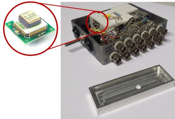
Figure 6. Accelerometer and Hall sensor assembly without the top cover
