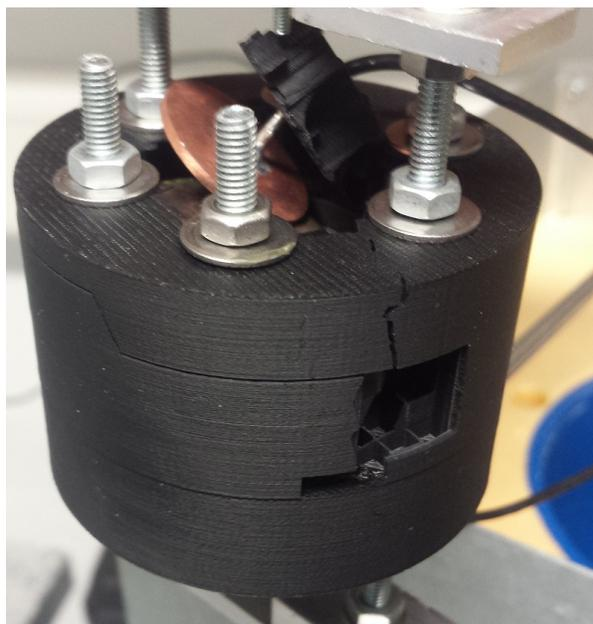
**Figure 12. The destroyed second support after a few discharges at  $1.3 \text{ kV}$  into the YBCO disc**
