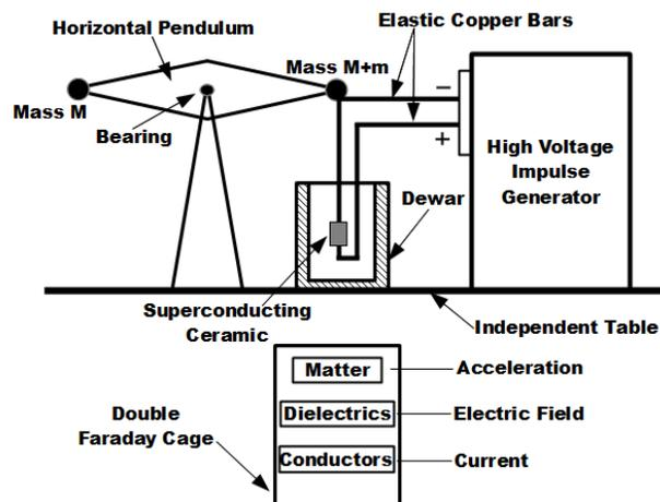
Figure 2. Schematic of Poher's Experimental setup and sensor arrangement<sup>11</sup>
