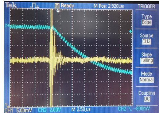
Figure 5. Induced EMP picked up by our oscilloscope. Channel 1 (5 mV/div) is measuring the output of an accelerometer, while Channel 2 (2 V/div) is measuring the output from the current sensor
