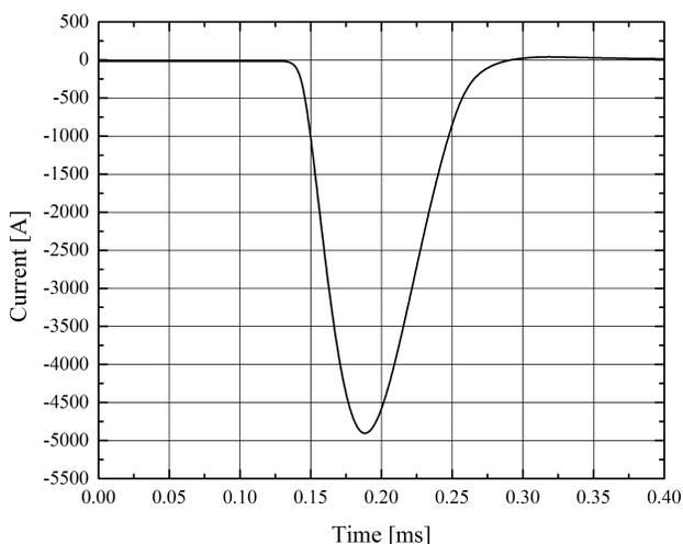
**Figure 11. Current impulse profile of a  $1.7 \text{ kV}$  discharge into a  $22$  diameter,  $3 \text{ mm}$  thick aluminum disc at room temperature**
