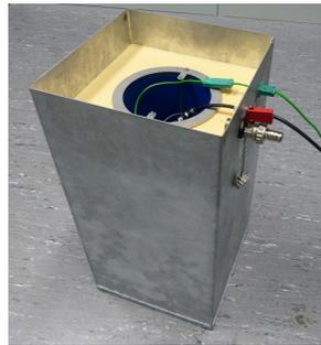
(b) Finished cryostat without its top cover
