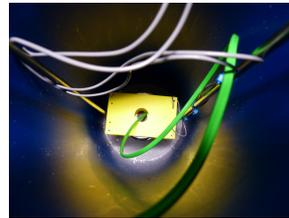
(c) Mounted HTSC disc at the center of the solenoid
