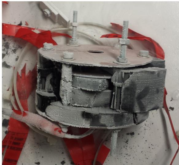
**Figure 16.** Destroyed support and superconductors by the double HTSC disc configuration during 1.7 kV discharges (photo taken right after the assembly was dismantled from the cryostat)
