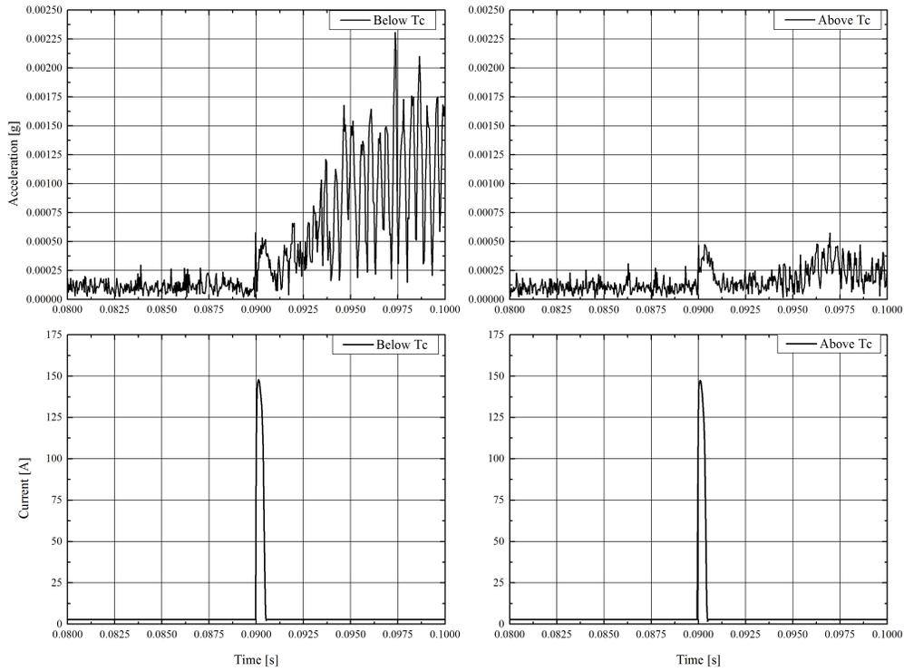
**Figure 8. Magnitude of the 3-D acceleration field change measured during 20 impulses and averaged in non-superconducting (right) and superconducting state (left) of the YBCO disc**
