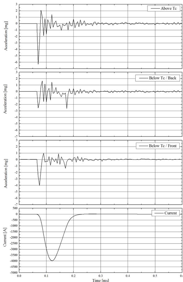
**Figure 13. Measurement results with the piezoelectric sensor during discharges of 1.2 kV into the 22 mm YBCO disc**
