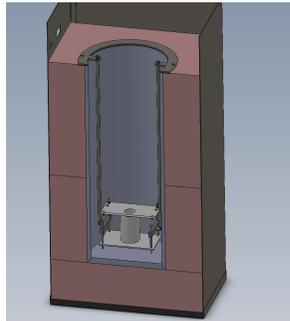
(a) Cryostat CAD model cross section
