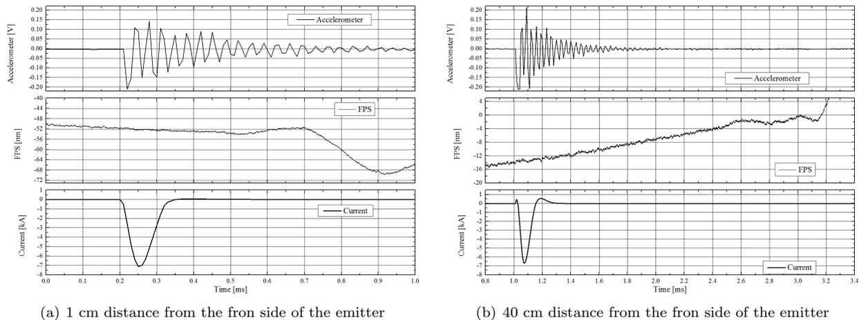
**Figure 15.** Representative measurements done with the optical accelerometer and piezo-accelerometer during discharges of 2.2 kV
