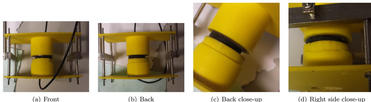
Figure 9. Broken HTSC disc support
