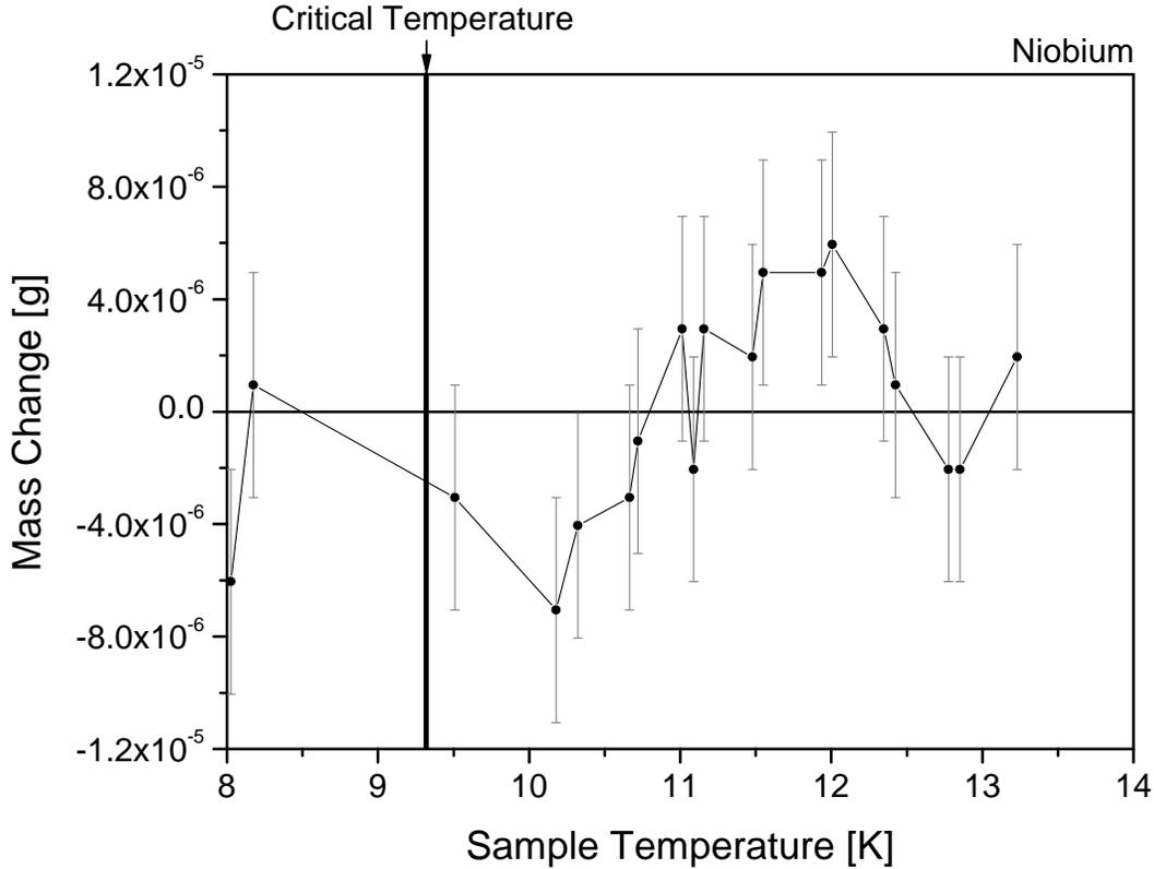
**Figure 8.** Mass Changes along Critical Temperature for Niobium Sample
