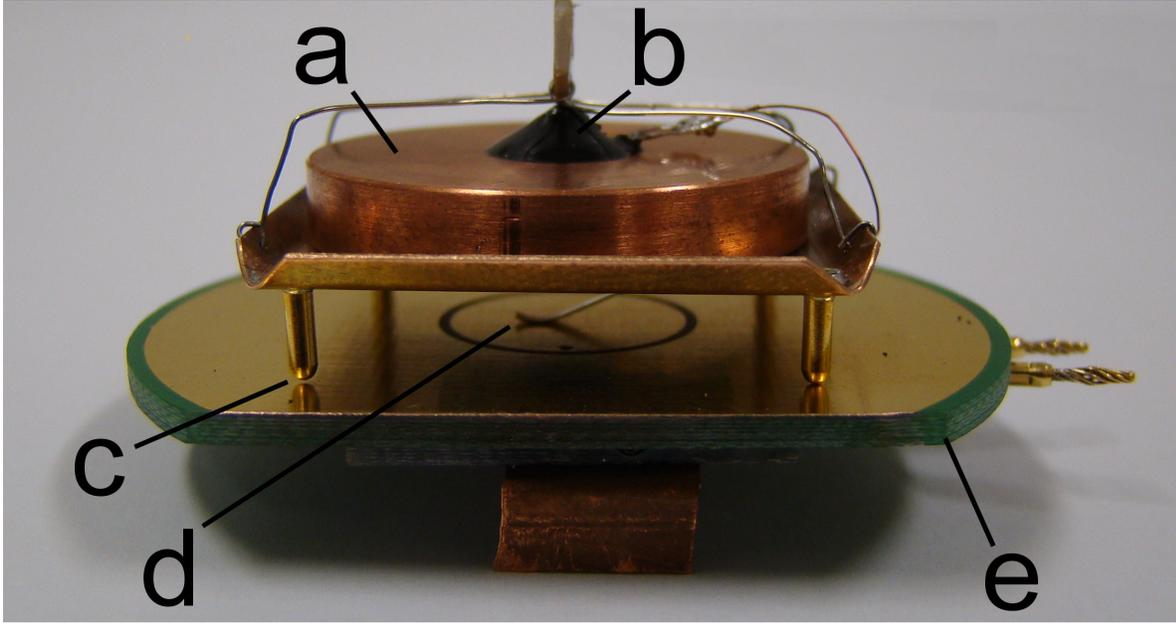
**Figure 3.** Details of the Sample Holder with Copper Sample (a ... Sample, b ... Silicon Diode, c ... Pin, d ... Spring Connector, e ... Connecting Plate)
