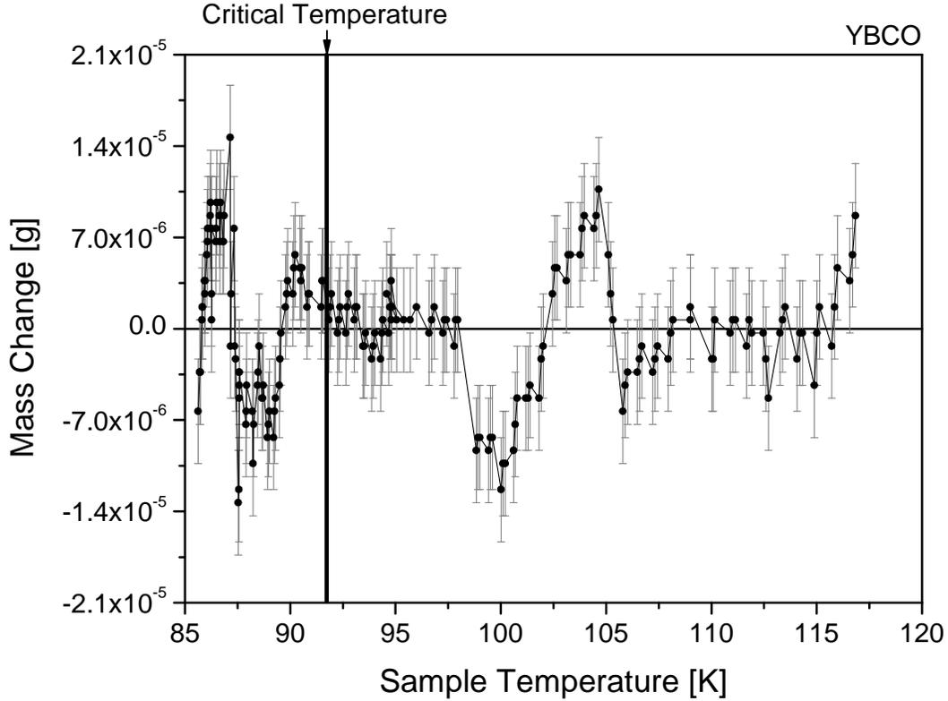
**Figure 7.** Mass Changes along Critical Temperature for YBCO Sample
