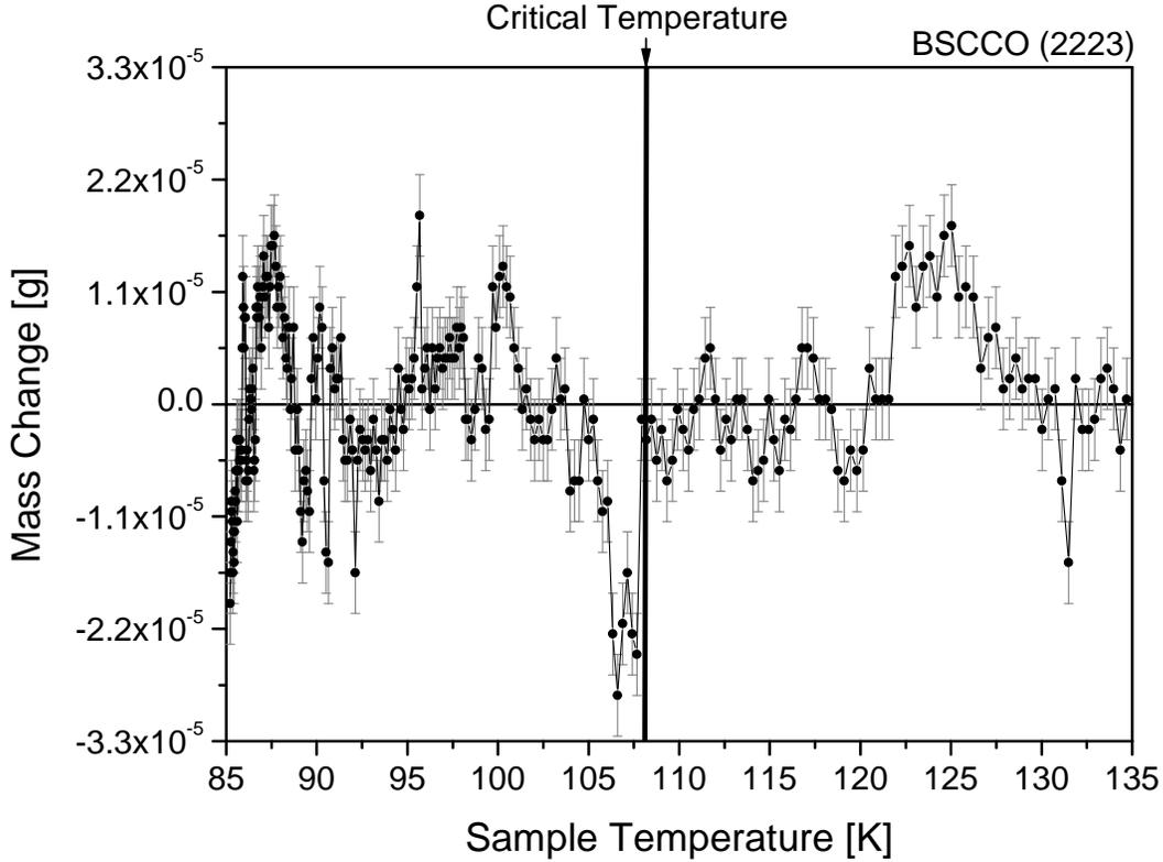
**Figure 6.** Mass Changes along Critical Temperature for BSCCO (2223) Sample
