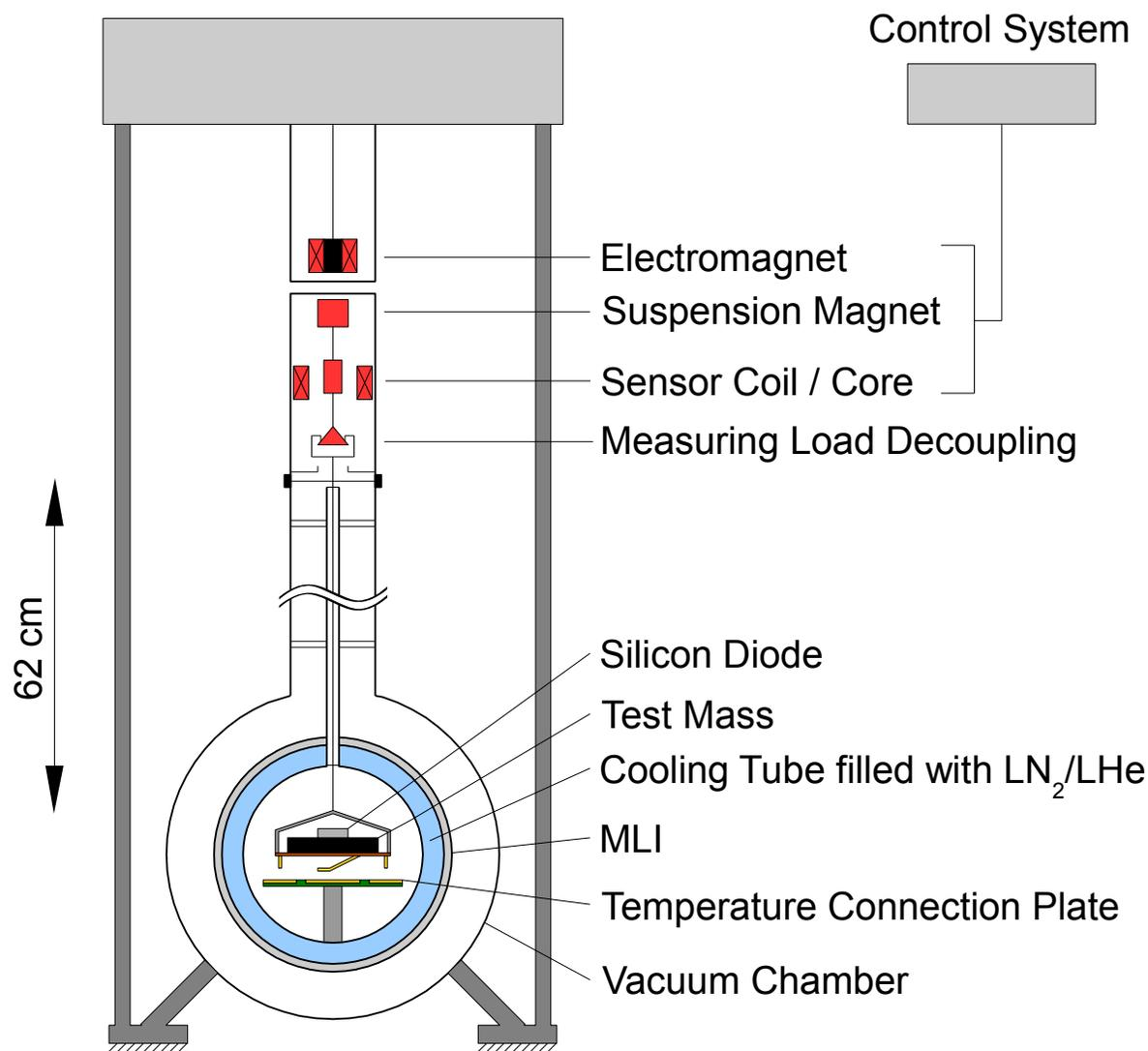
**Figure 1.** Experimental Setup
