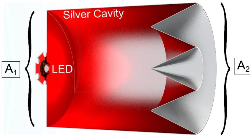
**Figure 6** Schematic Sketch of BART Drive in Sectional View (Rotationally Symmetric around Middle Axis) illustrating the Difference in Area  $A_1 < A_2$
