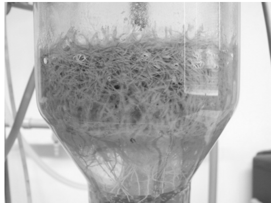
Fig. 2 Hairy root in bubble column bioreactor
