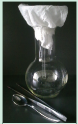
Fig. 6: Device for separation of plant cells from bacteria
