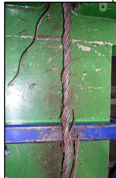
Rope test rig with three bending zones
