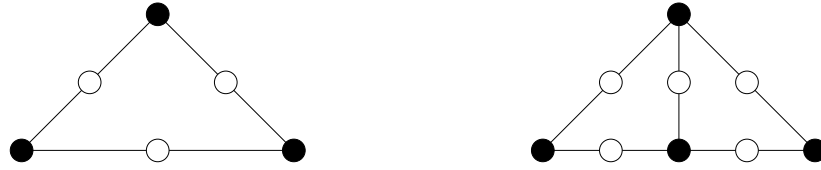
(a) DOF locations in the parent triangle. (b) DOF locations in the two child elements.
