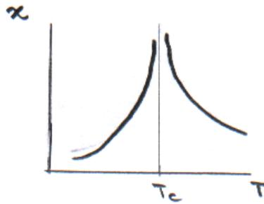
Figure 2.6: Singular behavior of the order-parameter susceptibility  $\chi$  near  $T_C$ . For ferromagnets, the behavior for  $T > T_C$ ,  $\chi = C/(T - T_C)$  with  $C$  the Curie constant, is also known as Curie-Weiss law.
