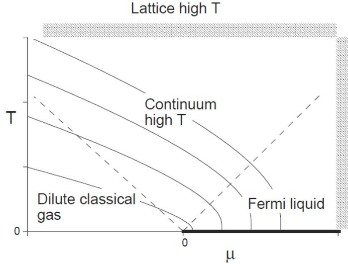
Figure 7.6: Phase diagram of the dilute Fermi gas as function of chemical potential  $\mu$  and temperature  $T$ . The QCP determining the structure of the phase diagram is at  $\mu = 0$ ,  $T = 0$ ; it is the endpoint of a critical line located at  $\mu > 0$ ,  $T = 0$  which controls the Fermi-liquid phase. The dashed lines mark the crossover  $T^* \propto |\mu|^{\nu z}$  with  $\nu z = 1$ ; the solid lines denote lines of constant density. Figure taken from [1].
