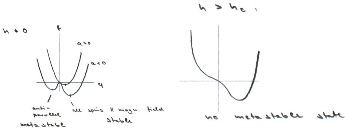
Figure 2.5: Landau potential  $f$  (2.2) for  $h \neq 0$ , displaying minima which correspond to either stable or metastable states.
