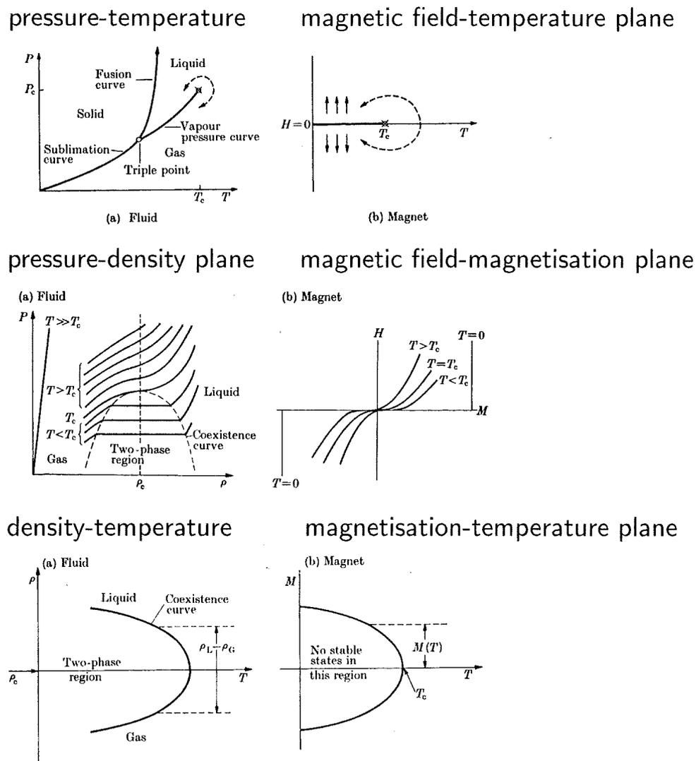
Figure 2.2: Different representations of the generic phase diagrams of (a) fluids and (b) magnets.
