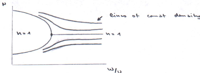
Figure 7.4: Lines of constant boson density  $\langle n \rangle$  in the phase diagram of the Bose-Hubbard model.
