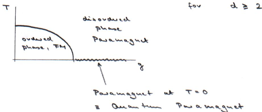
Figure 4.2: Finite-temperature phase diagram of the quantum Ising model.
