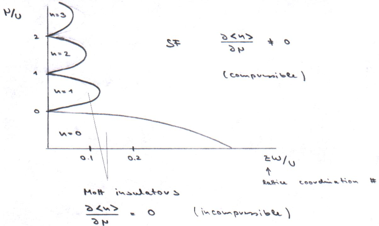
Figure 7.3: Mean-field phase diagram of the Bose-Hubbard model as function of  $\mu/U$  and  $zw/U$ , showing Mott and superfluid phases.
