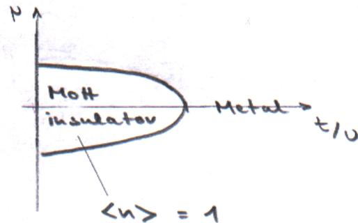
Figure 7.7: Simplified generic phase diagram of the Hubbard model. Symmetry-broken states (magnetic, superconducting, etc.) are not shown.
