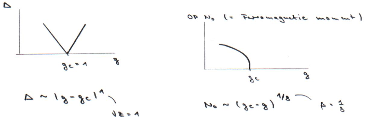
Figure 6.10: Excitation gap and ferromagnetic moment (order parameter) of the quantum Ising chain near criticality.
