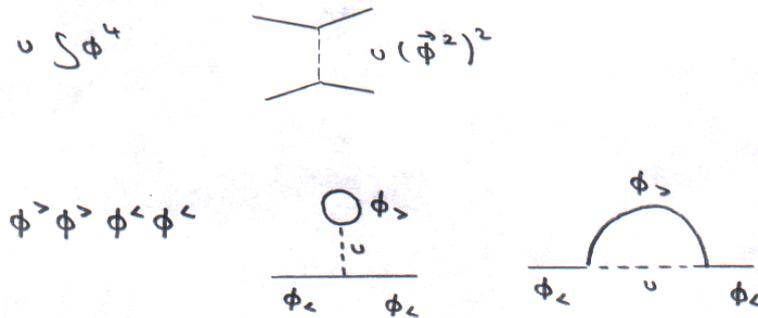
Figure 3.4: Top: Graphical representation of the quartic interaction. Bottom: Feynman diagrams to linear order in  $u$  – both induce a renormalization of the coupling constant  $r$ .
