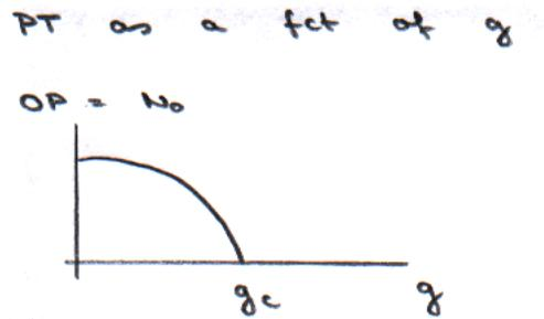
Figure 4.1: Order parameter of the quantum Ising model as function of the tuning parameter  $g$ .
