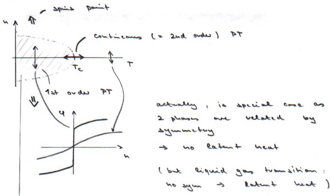
Figure 2.8: Continuous and first-order transitions in the temperature–field phase diagram of a magnet as described by Landau theory.
