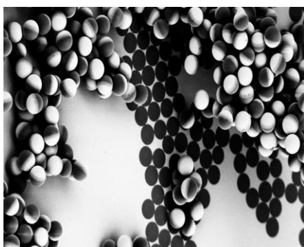
Electron microscope image of nanoscale Janus particles, which the Freigeist group is going to test regarding their capacity as photocatalytic nanomotors. Credits: Juliane Simmchen
